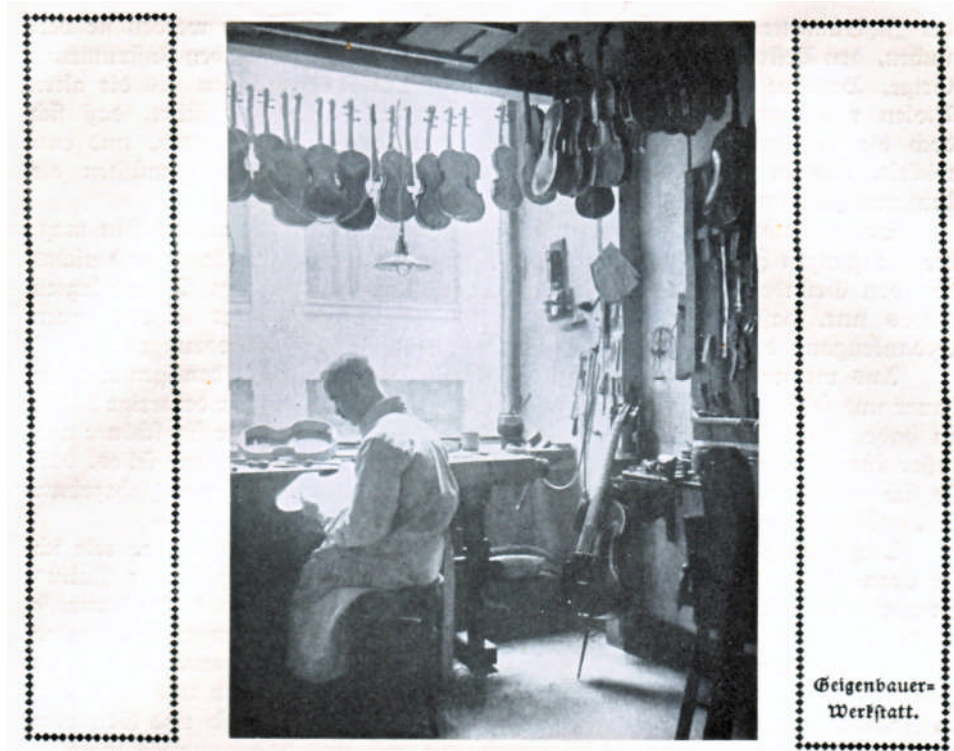
Figure 1: ‘Violin maker’s workshop’ from R. Möller Laute, Viola da gamba, Viola da braccio , p. 19. At the rear left the body of a viol to Möller’s design (see Figure 2) may be seen, on the right a small bass viol in ‘violin’ form.
