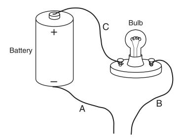
The bulb is **not** lit. What should be done in order to light the bulb and complete the circuit?
