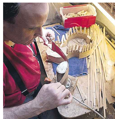
A small heater is used to shape lining strips for the inside edge of an instrument's rib.
