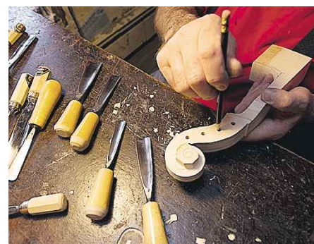
A handful of woodworking tools are needed to create a scroll for a new violin.
