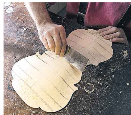
The back of a violin is shaped with a miniature flat plane.
